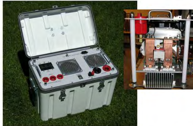
KMS-5100 land EM transmitter in portable field box, inside view. Timing and system response controller, and optional shock mounted, dustproof case.
